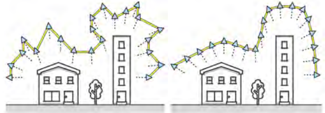
Fig. 2. An illustration contrasting a shortest path constructed from independently selected good viewpoints (left) vs. an aerial path computed using our continuous planning approach (right). Our path on the right is optimized to have fewer sharp turns while ensuring a good view coverage of the scene.
